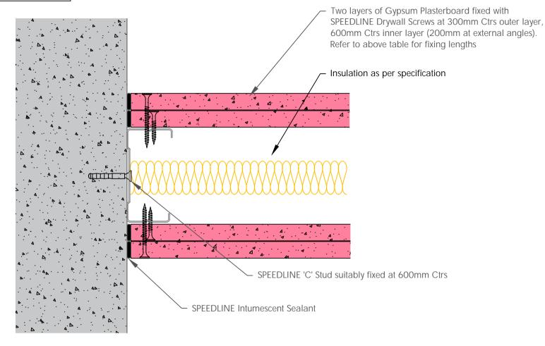
All performance data and system specifications are for systems constructed with materials & components as shown. The inclusion or substitution of any other manufacturers material or components could invalidate test data and system performance and permission must be given in writing by SIG FLC.
